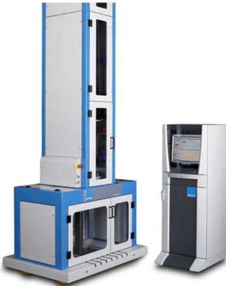
A highly versatile range of drop weight impact testers for performing a wide range of medium energy tests on materials, specimens and end products of various geometry.
